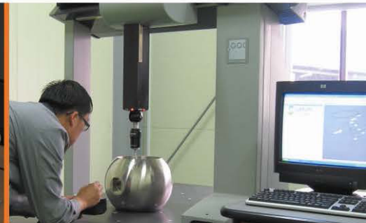
Ball testing by 3D measurement
